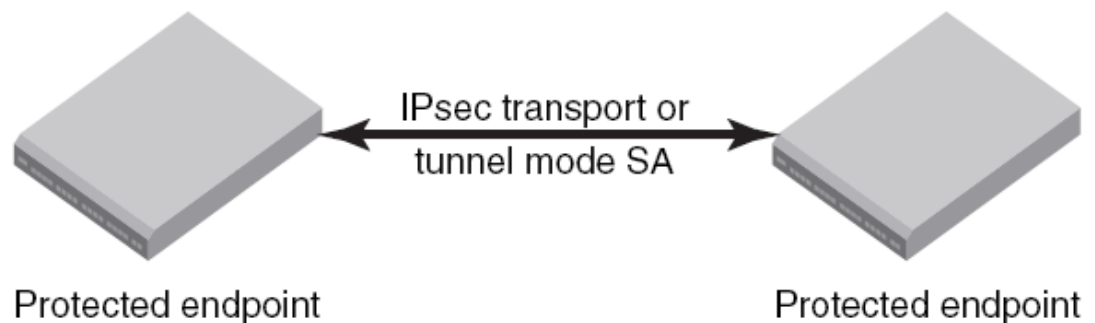
FIGURE 18 Protected endpoints configuration
